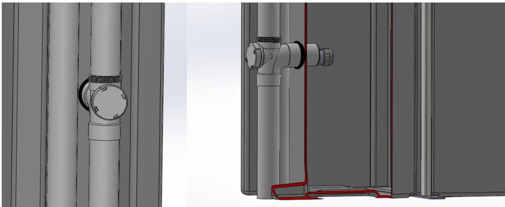
**\*Warning\*** Correct hole saw sizes must be used for the wallace seals provided to avoid leaks.
