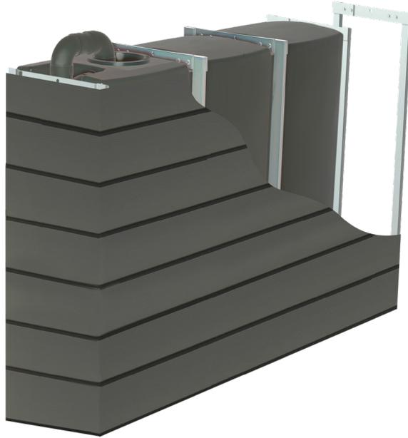
Tec screws can be used to attach timber/panels etc to the steel frames. Ensure that the correct length screws are used to avoid going through the steel and into the tank. No more than 20mm longer than the thickness of whatever is being attached.
