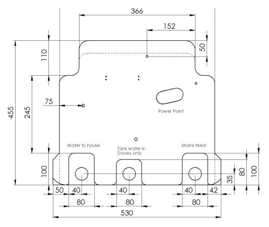
\*\* Screw locations should be kept within the dotted area above when fixing to wall.
