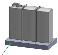
Seismic base slab
